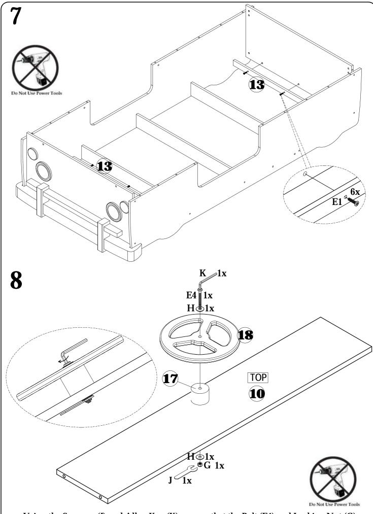
Using the Spanner (J) and Allen Key (K), ensure that the Bolt (E4) and Locking Nut (G) are securely fixed and that the wheel can still turn freely.
