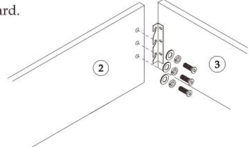
Before tightening the bolts, please ensure the bed frame is square.
