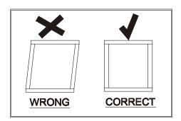
Fix corner brackets, then repeat for other 3 corner brackets in each corner of the bed frame.
