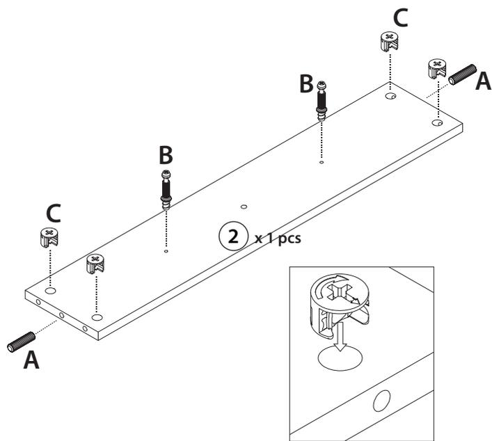
Proper orientation of CAM LOCK
