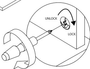
Tighten the cam locks clockwise.
