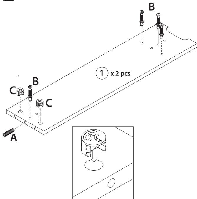
Proper orientation of CAM LOCK
