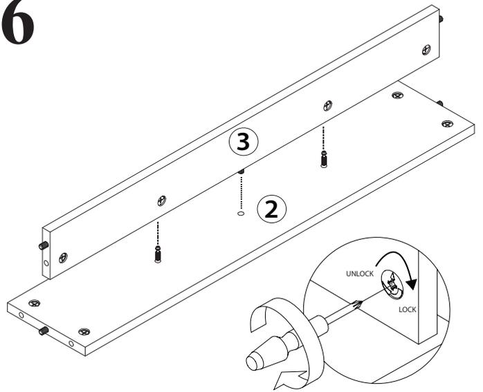
Tighten the cam locks clockwise.
