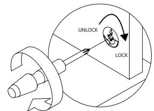
Tighten the cam locks clockwise.
