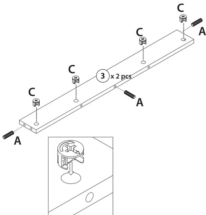
Proper orientation of CAM LOCK
